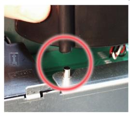
Be sure you set the fan on the mounting pins, as shown above.
